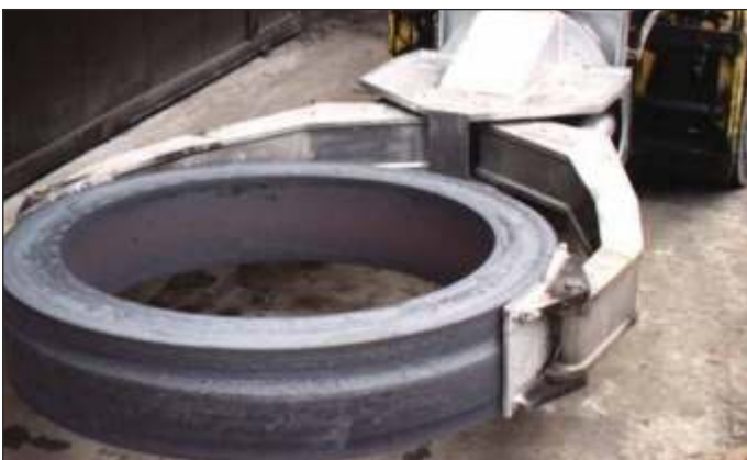
FORGING MANIPULATOR AND CLAMP Safe Loading of Furnaces and Forging Presses
