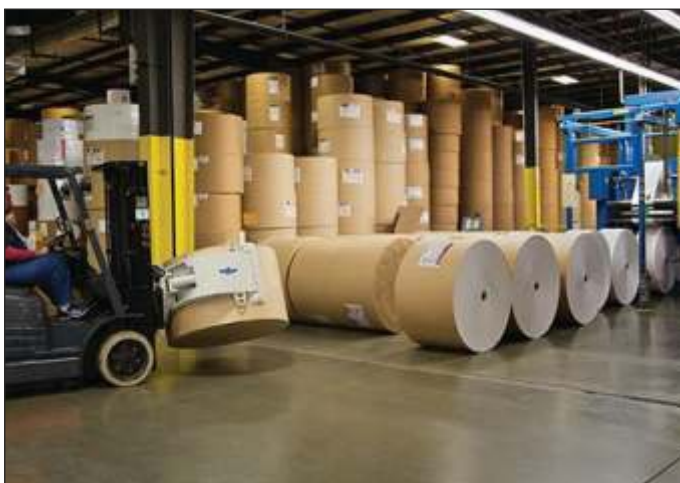
13H PAPER ROLL CLAMP Specifically designed for printers and newspaper publisher.
